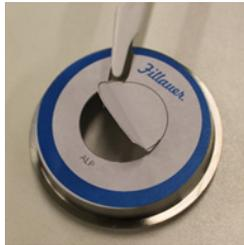
3. Flip the adapter and insert the washer with the protruding stud facing down into the hole, according to the picture.
