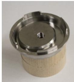
4. Place the sealing washer in the lamination adapter and seal the edges with a narrow strip of silicone seal. Wacker Elastosil E43 is recommended, Part nr. 632040090.
